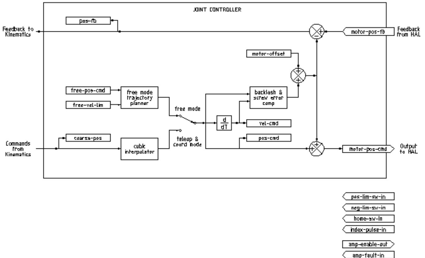
Figure 3.1 - Joint Controller Block Diagram
